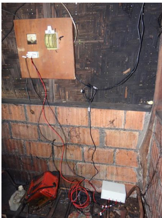
Figure 34: Load measurement LAE 1 at Generator #18
