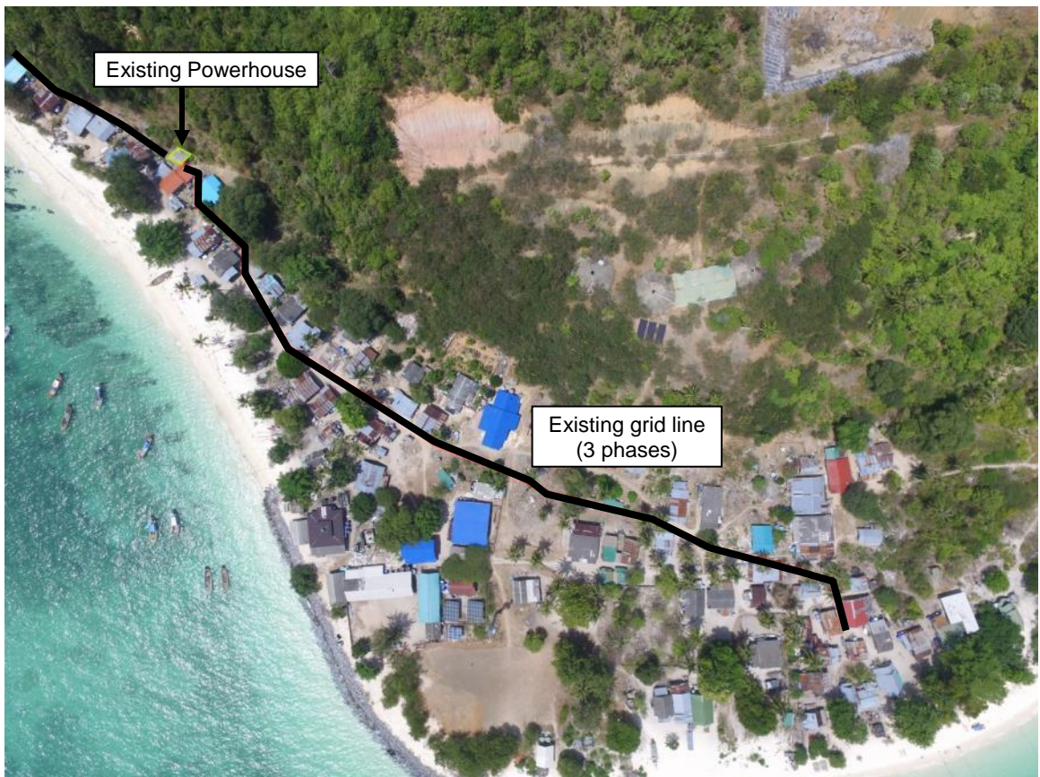
Figure 27: Existing central grid transmission route
