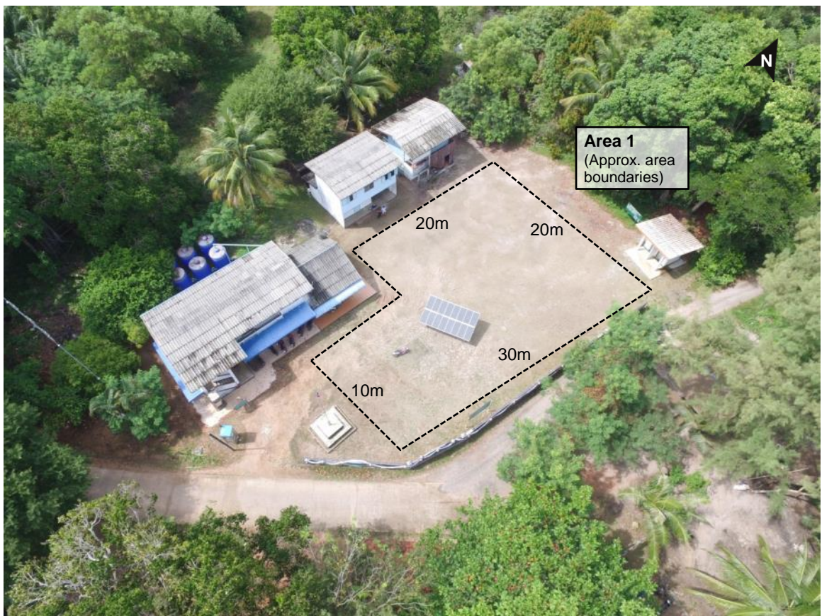
Figure 35: Possible area to install new a PV system at public health centre (Area 1)
