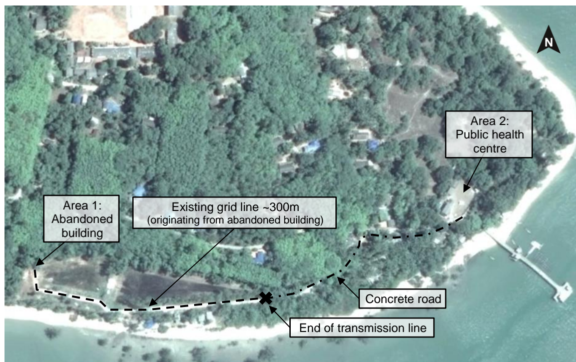
Figure 31: Two possible locations for new power house
