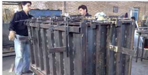
Figure 2: Foaming mould of the cabinet at Freidooni
